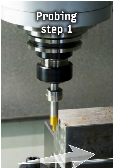
1. The edge finder body can be slipt out from the axis' centre by a gentle tip of the finger and is out-of-the-round.
